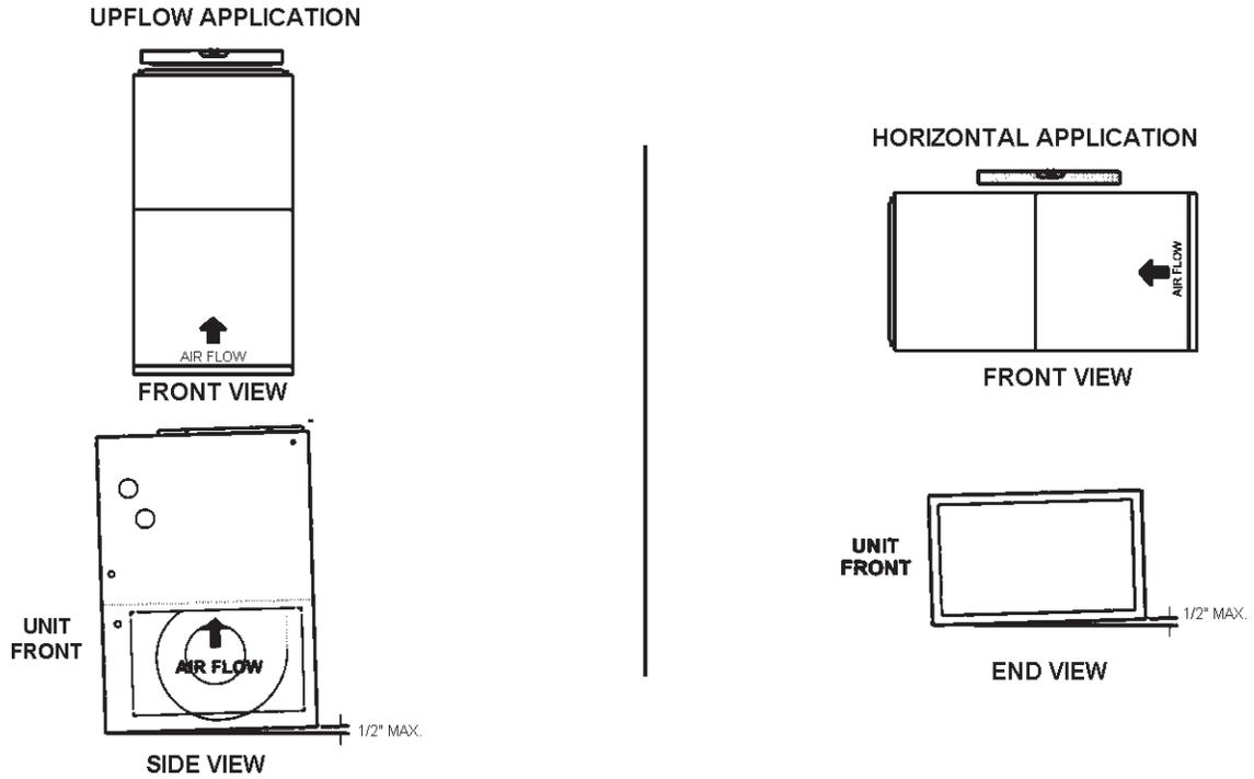
TILT THE UNIT SLIGHTLY (MAX. 1/2") FROM BACK TO FRONT TO AID IN THE DRAINING OF THE HEAT EXCHANGER.
