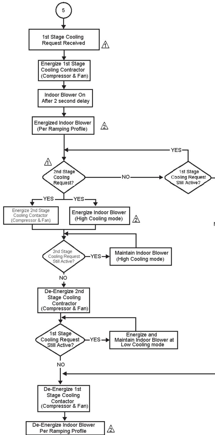
⚠ 2nd stage cooling operation requires a 2 stage thermostat, a 2 stage cooling system and on board link W915 must be cut. The control will not respond to a 2nd stage cooling request unless a 1st stage cooling request is active.
