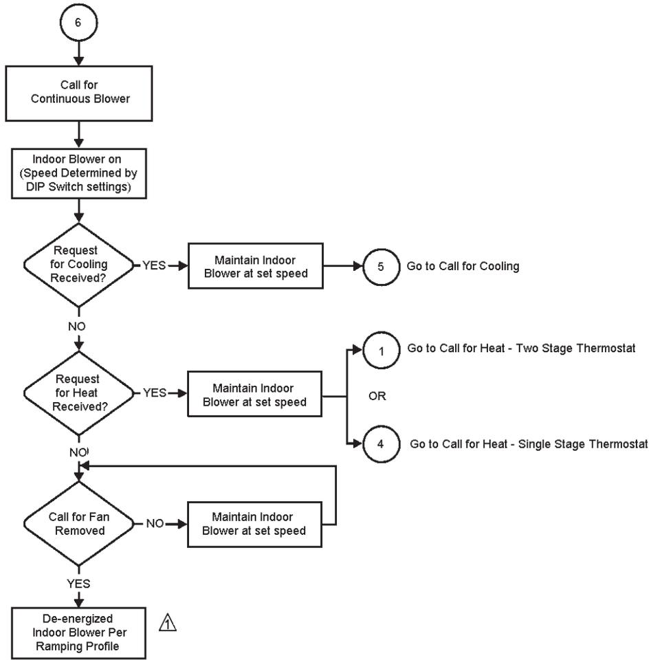
⚠ Indoor blower low cooling mode and high cooling mode, have specific ON - OFF and speed ramping profiles. The specific profile is selected using the DIP switches on the control.
